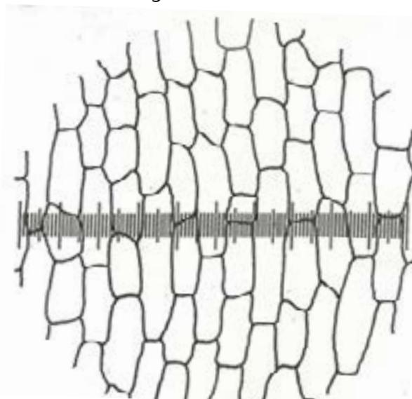
View at x400 of a plant tissue through an eyepiece containing a graticule scale
