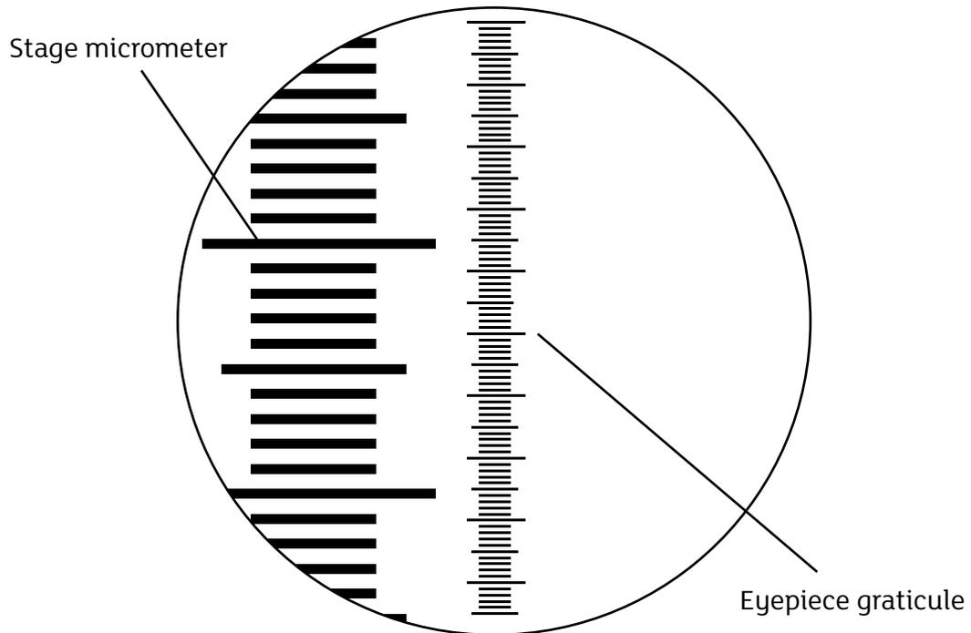
*Calibrating the eyepiece graticule at high power*
