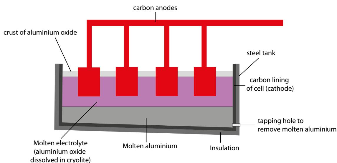
The alumina obtained from the purification has a very high melting point around 2050 °C. This is too high a temperature to make the process economically viable so it is dissolved in molten cryolite which reduces the temperature needed to melt the mixture to approximately 950 °C and also increases its electrical conductivity. A crust of aluminium oxide forms on the surface of the electrolyte which prevents heat loss reducing the energy cost of the process.
