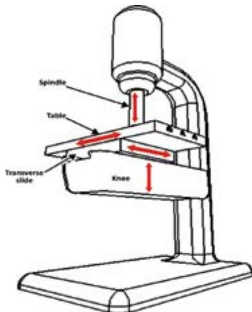
To cut a slot in the centre of a 25mm wide steel strip with a 6mm cutter, first touch on to the edge of the strip and set the read out to zero. Raise the cutter and move it a distance equal to half the diameter of the cutter plus half the width of the steel strip which in this example equals  $12.5 + 3$  (15.5mm).
