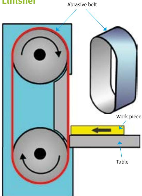
A linisher turns a belt of abrasive material which is used to smooth a workpiece, creating a level, even surface. Materials that can be used on a linisher are usually wood or metal.
