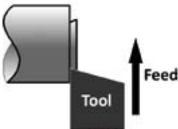
Facing produces a flat face at the end of the part which is perpendicular to the axis of the machine.
