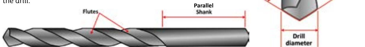
Large diameter drills generally above 13 mm have a taper shank to ensure correct alignment of the drill. The tapered section fits into the spindle of the drilling machine or tail stock of a lathe and locks in position. The taper used is called a morse taper and is self-locking in that it will grip and hold in position and must be removed from the spindle by using a wedge called a drift to release the taper.
