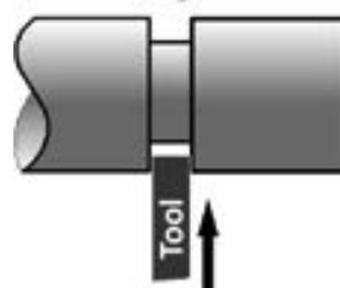
Parting is a process which removes a piece of material from the end of a longer bar. The piece removed may be a completed part or a blank to be used in further processing.
