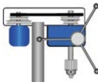
The drill is driven by a stepped cone vee belt drive which can deliver three or four drill speeds. Small diameter drills need to run at the highest speed and large diameter drills at slower speeds.
