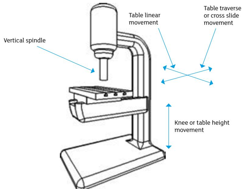
Milling is a machining operation that uses a rotating cutter to remove material from the work piece. There are two main groups of milling machine, those with a vertical spindle and those with a horizontal spindle. A vertical milling machine is shown. The cutter rotates in a fixed position and the work piece is bolted to the machine table or held in a sturdy machine vice.
