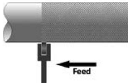
Knurling produces a regular roughened surface on cylindrical surfaces to provide grip on knobs and handles.
