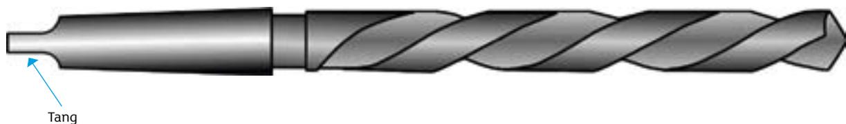
The taper shank drill has a tang on the end of the taper to ensure a positive drive from the spindle of the drilling machine.
