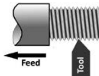
Screw cutting uses the feed mechanism to cut a specific pitch of thread with a precise tool ground to the correct angle. Internal and external threads can be cut on a lathe.
