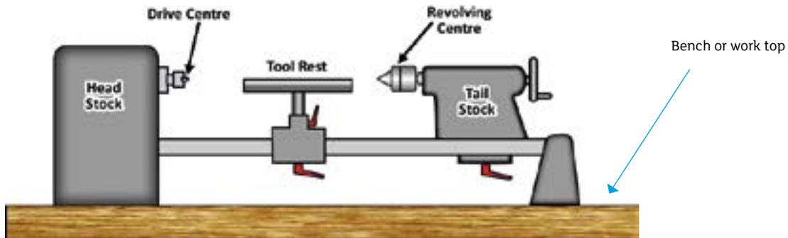
The work rotates towards the user. The tool rest is set close to the work piece and the chisel is held firmly up to the work.
