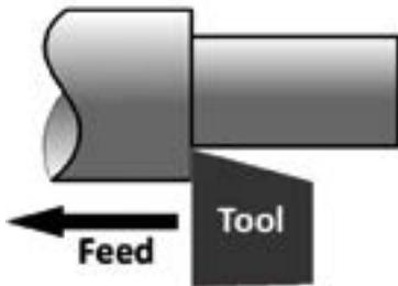
To produce parallel shafts and to reduce the diameter of the work piece.
