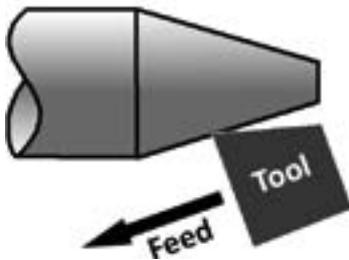
To cut a taper the compound slide must be set and locked in the required position. The compound slide hand wheel is used to move the tool and cut the taper.
