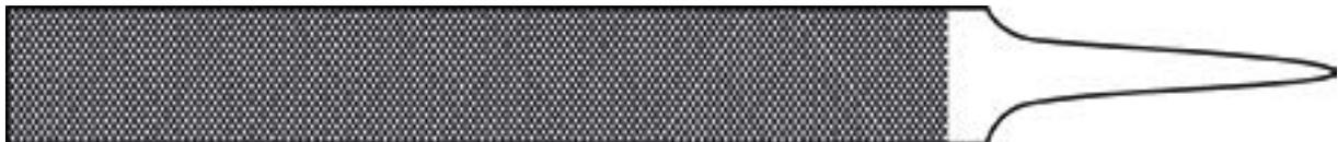
Files are made from high carbon steel which is hardened and tempered and have a tapered end called a tang onto which a wooden handle is fitted. The faces of the file have groves cut into them to form the teeth of the file.
