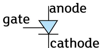
A thyristor is a semi-conductor device. It is triggered to conduct a forward current (in the direction of the diode arrow – from the anode to the cathode) if a small trigger pulse of current is detected at the gate.
