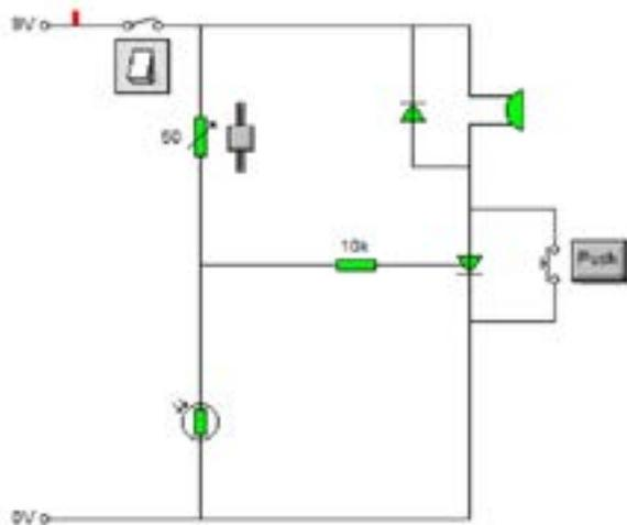
When the SPST is closed and in dark conditions the LDR will have a high resistance, this will cause a small voltage at the gate of the thyristor; the thyristor will then be turned on, allowing current to flow from the anode to the cathode. The buzzer will sound.
