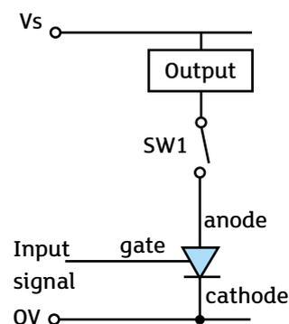
The circuit on the left will switch the current through the output device on if the switch SW1 is closed and the Input signal voltage (applied to the gate) is detected.
