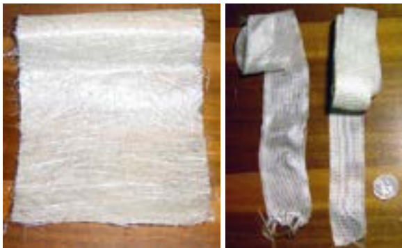
A roll of Chopped Strand Mat (left) & (right) two rolls of Plain Weave Cloth tape.
