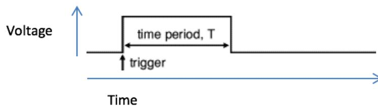
This waveform represents what is happening at Pin 3, once the switch is pressed. pin 3 immediately goes high for a period of time (T) and then returns to low again.
