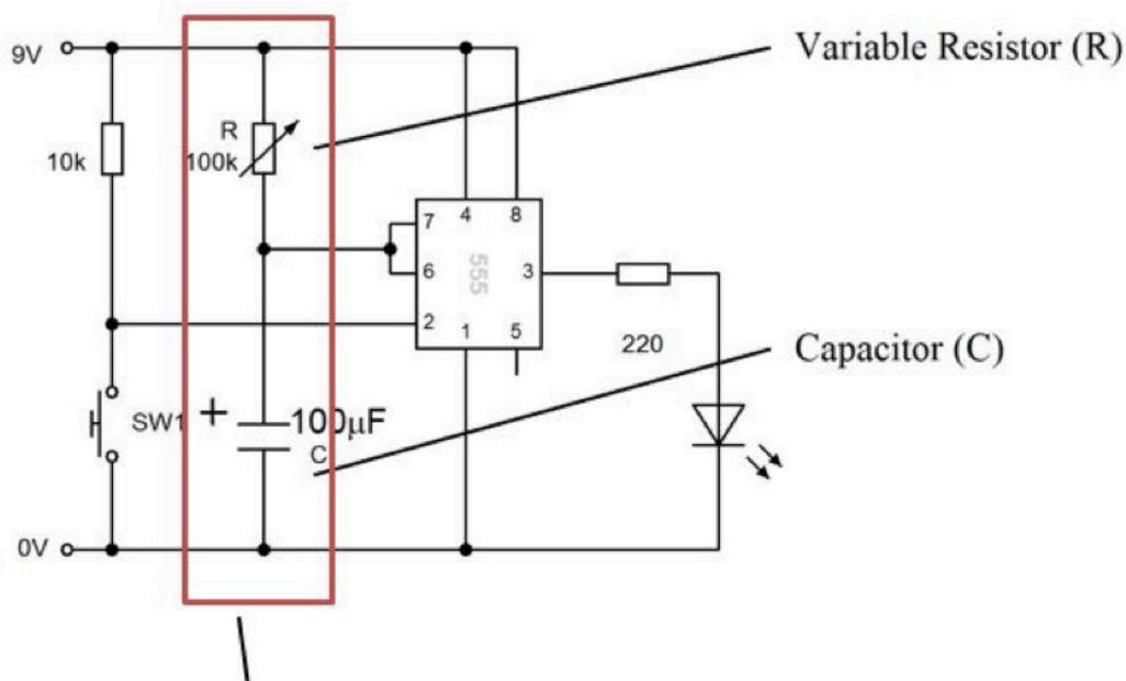
The section above is called the RC network; it has a resistor (in this case a variable resistor) and a capacitor in series.
