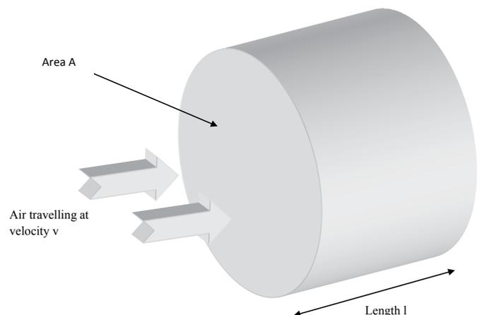
The energy available from the wind is due to its kinetic energy which is given by the equation;
