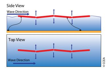
As the cylindrical parts follow the motion of the waves they drive hydraulic rams in the various sections which are connected together, which in turn drive electrical generators. The electricity can then be combined from the different sections of the structure and sent to the shore via a cable. Further information on Pelamis can be obtained at; www.pelamiswave.com
