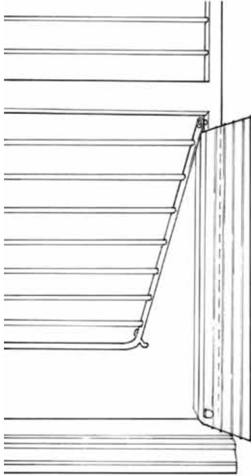
The rubber ramp is placed on top of the bottom bar of the child safety gate and provides a safe and smooth ground-to-sill transition.
