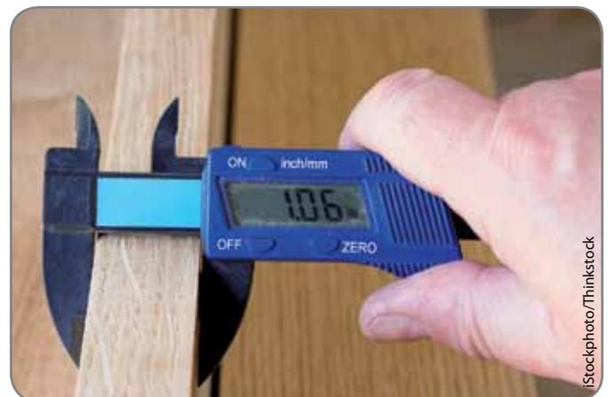
Tolerances provide the maximum (+) and minimum (-) deviation from the actual value that will still allow it to do its job.
