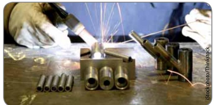
**Oxy-acetylene:** For this method acetylene is burned with oxygen to produce a heat source of approximately 3500°C. Fine adjustment of the gases can be made by the user altering the gas feed on the handle of the torch.
