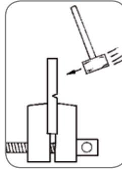
The amount of energy that can be absorbed during fracture also depends on the size of the piece of material, therefore in the IZOD test, the different materials must be the same size.
