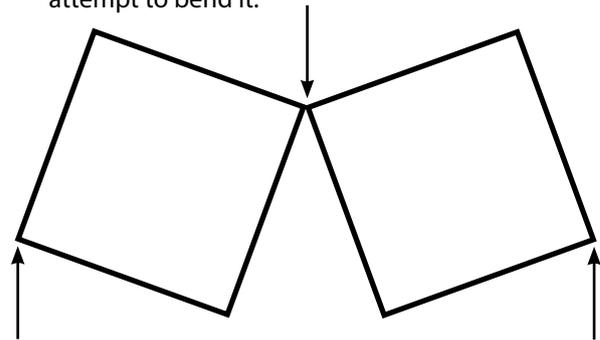
4. **Shear force** is the force that subjects materials to a sliding action across their surfaces. This kind of force is present in hinges, rivets, scissors, secateurs for gardening, manual hedge clippers and other tools that involve two or more blades sliding across each other.
