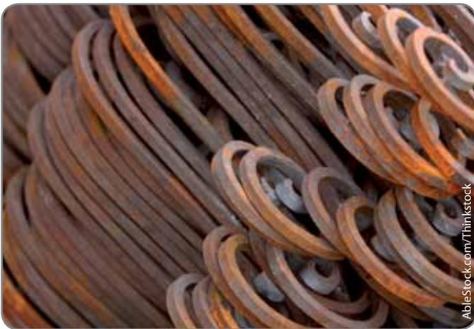
Ferrous metals such as steel and cast iron are graded by size prior to being melted down. They have a relatively low scrap value and this can be an issue as it could be more economical to use steel produced from raw materials as opposed to using steel made from scrap. Although there is a case against the recycling of steel on economic grounds it is the world's most recycled material.
