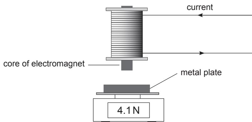
An experiment is carried out to investigate how the strength of the electromagnet depends on the current in the coil.
