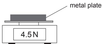
The electromagnet is placed above the metal plate as shown below. When the electromagnet was energised by passing a current through the coil an upward force was exerted on the metal plate. This reduced the reading on the electronic balance.
