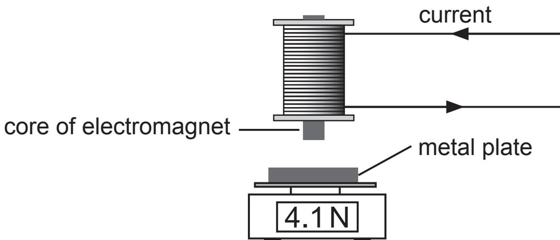
An experiment is carried out to investigate how the strength of the electromagnet depends on the current in the coil.
