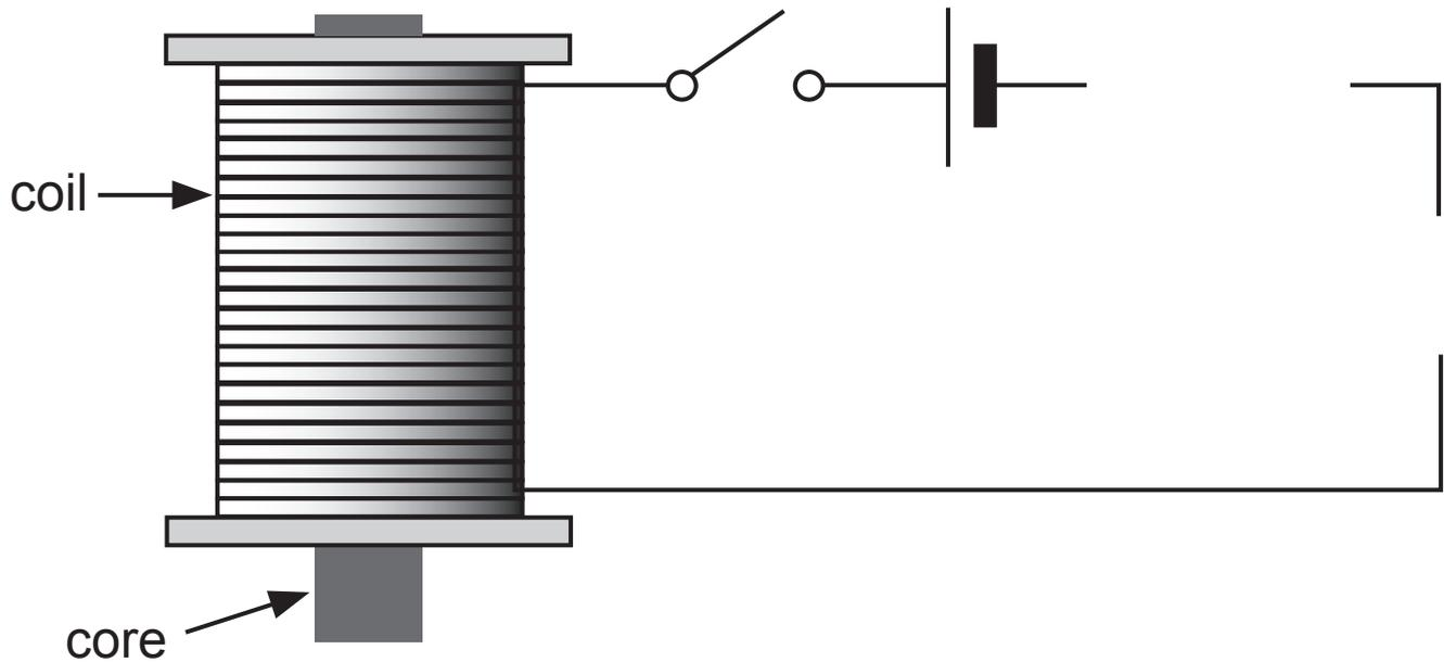
When an electric current flows through the coil the metal core becomes an electromagnet.
