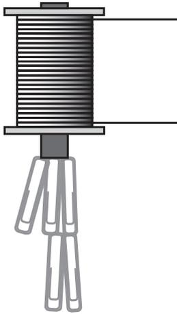
The maximum number of paper clips that the electromagnet could lift was counted for each value of the current.
