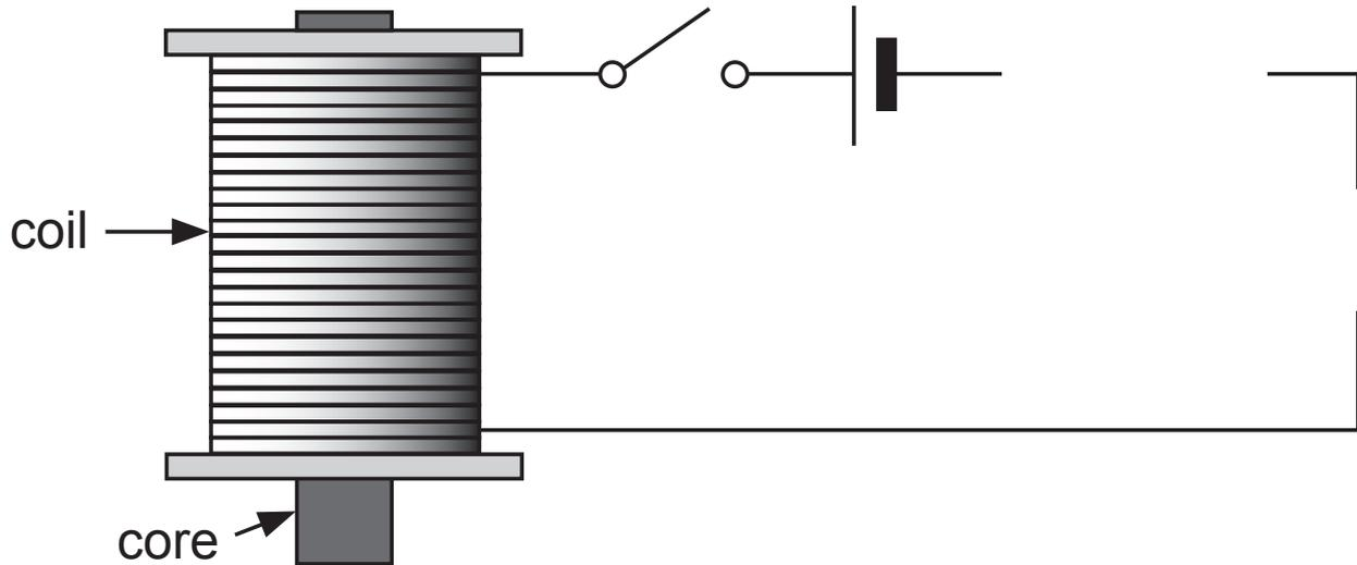
When an electric current flows through the coil the metal core becomes an electromagnet.
